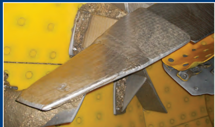
Rex Hurricane Style mixing blades that have been in service for 720,000 yards.
