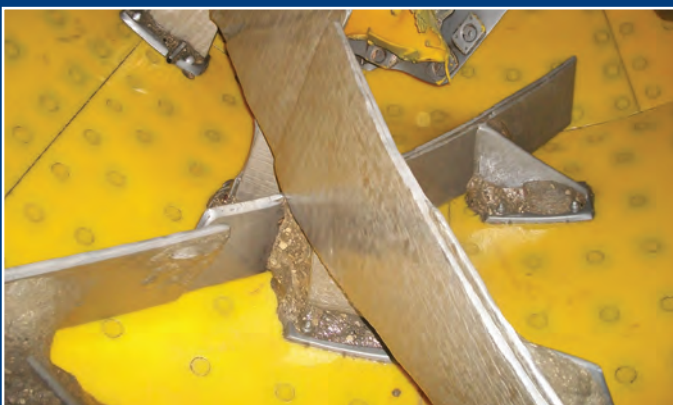
Rex Hurricane Style mixing blades that have been in service for 720,000 yards.
